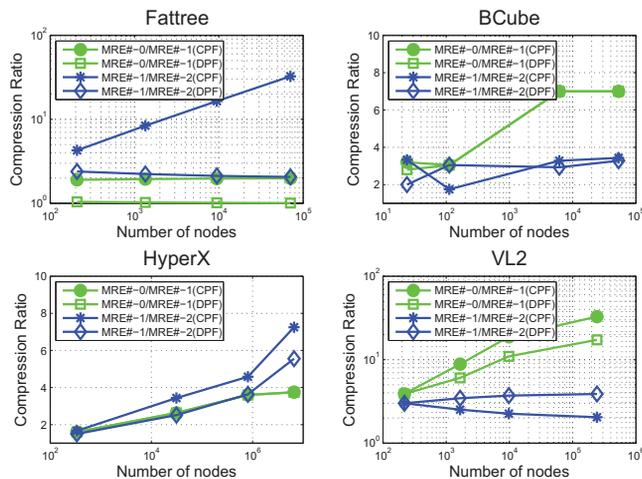
Fig. 7. CPF vs DPF: the compression ratio of maximum routing entries without compression to maximum routing entries after Step I compression (MRE#-0/MRE#-1) and the compression ratio of maximum routing entries after Step I compression to maximum routing entries after Step II compression (MRE#-1/MRE#-2).
