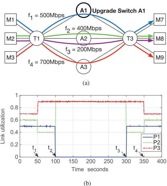
Fig. 14. XPath utility case #2: we leverage XPath to assist zUpdate [28] to accomplish DCN update with zero loss. (a) Path  $P_1$ :  $T1 \rightarrow A1 \rightarrow T3$ ;  $P_2$ :  $T1 \rightarrow A2 \rightarrow T3$ ;  $P_3$ :  $T1 \rightarrow A3 \rightarrow T3$ , (b) Time  $t_1$ : move  $f_3$  from  $P_2$  to  $P_3$ ;  $t_2$ : move  $f_1$  from  $P_1$  to  $P_2$ ;  $t_3$ : move  $f_1$  from  $P_2$  to  $P_1$ ;  $t_4$ : move  $f_3$  from  $P_3$  to  $P_2$ .
