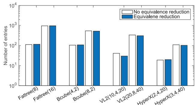
Fig. 6. Effect of ID assignment algorithm with and without equivalence reduction for the 4 DCNs.
