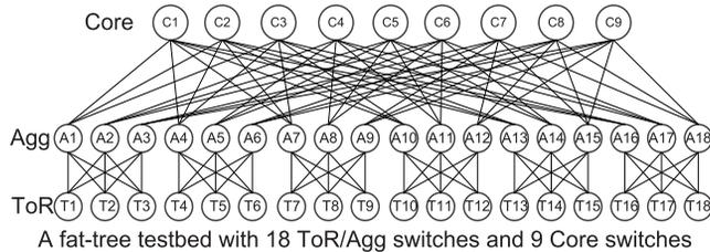
Fig. 9. Fattree(6) testbed with 54 servers. Each ToR switch connects 3 servers (not drawn).
