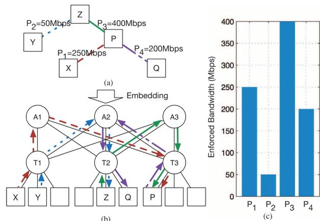
Fig. 15. XPath utility case #3: we leverage XPath to accurately enforce VDC with bandwidth guarantees.
