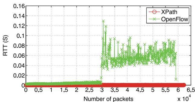
Fig. 12. Pre-installation under XPath vs dynamic installation under OpenFlow as packet/flow increases.
