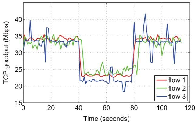
Fig. 11. TCP goodput of three connections versus time on three phases: no failure, in failure, and recovered.
