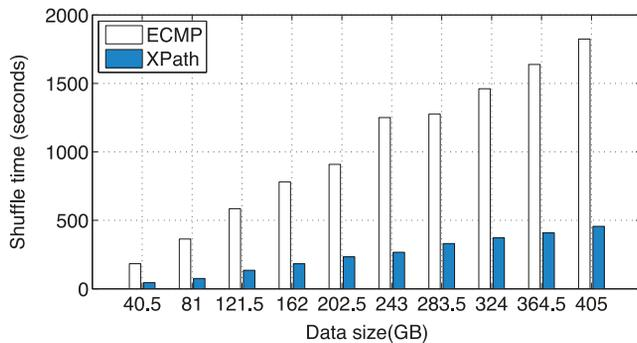
Fig. 16. XPath utility case #4: we leverage XPath to select non-conflict paths to speed up many-to-many data shuffle.
