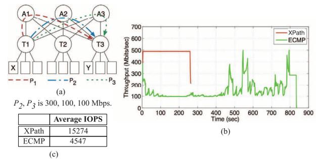
Fig. 13. XPath utility case #1: we leverage XPath to make necessary bandwidth easier to implement for provisioned IOPS.
