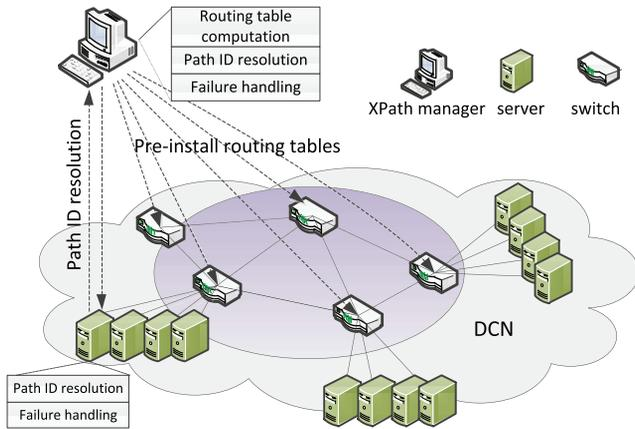
Fig. 2. The XPath system framework.
