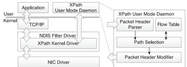
Fig. 8. The software stacks of XPath on servers.
