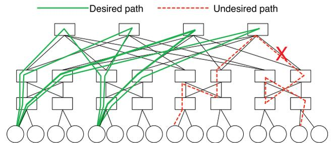
Fig. 1. Example of the desired paths between two servers/ToRs in a 4-radix Fattree topology.
